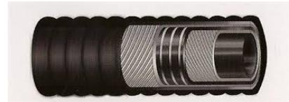
Tube: Heavy abrasion resistant black synthetic rubber. High tenacity canvases inserted. Built-in steel spiral. External surface with wide corrugation and canvas impression.
