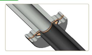
**CORRECT** on raised-face flanges with carbon fibre gasket
