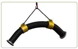
For transportation, installations or support in place, never use a single rope to lift hose. Only slings in sufficient numbers depending of the hose lengths.
